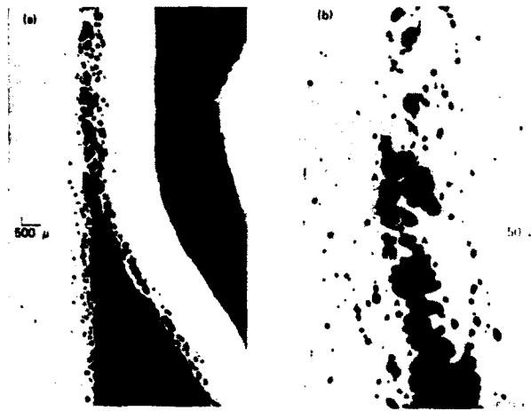
Fig. 1. A sample of full separation of an aluminum target. Impact test performed by Seaman et al. [25].
